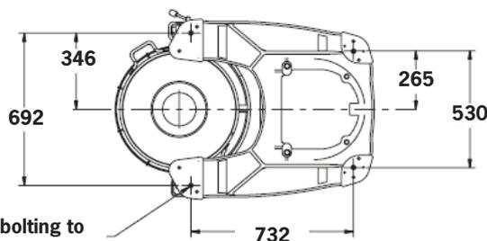
15.8mm dia. holes for bolting to floor (must be bolted to level floor)
