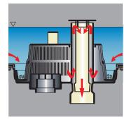
The original MEIKO eco-filter system filters the wash water in *UPster* machines, ensuring maximum hygiene and clean tank water.
